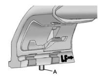
The crossrail supports are labeled with an arrow that needs to point toward the front of the vehicle. A pin (A) will be visible on the bottom when the crossrail support lever is down. To install the crossrail support, move the lever into the forward upper position, the pin (A) will not be visible.
